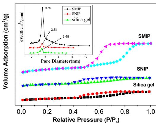
Fig. 5: Adsorption-desorption isotherms of nitrogen for silica gel, SNIP and SMIP
