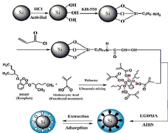
Fig. 1: The schematic illustration of synthetic route for SMIP.
