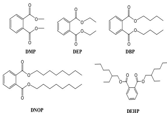
Fig. 2: Chemical structure of DEHP and its analogues.
