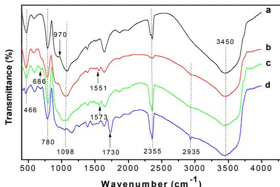
Fig. 3: FT-IR spectra of activated silica gel (a), ammoniated silica gel (b), acylated silica gel (c) and SMIP (d).
